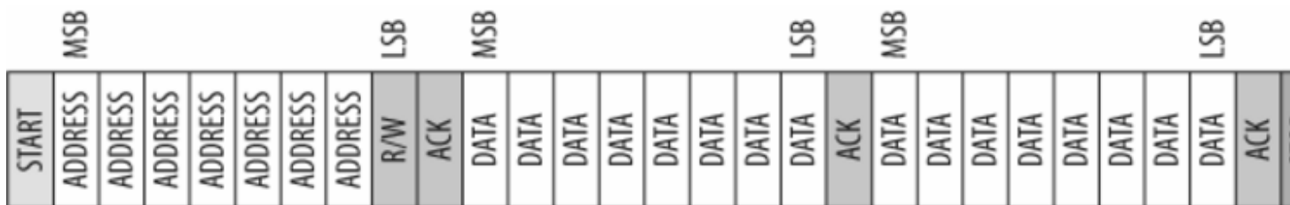
Figure 13-2. Format of a transaction on an I C bus
