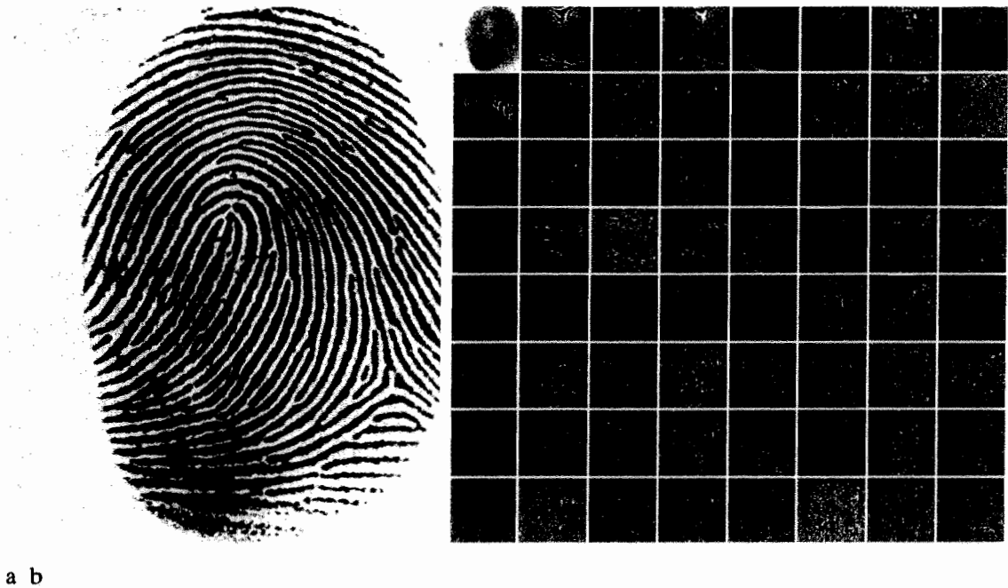
FIGURE 7.36 (a) A scanned fingerprint and (b) its three-scale, full wavelet packet decomposition. (Original image courtesy of the National Institute of Standards and Technology.)
