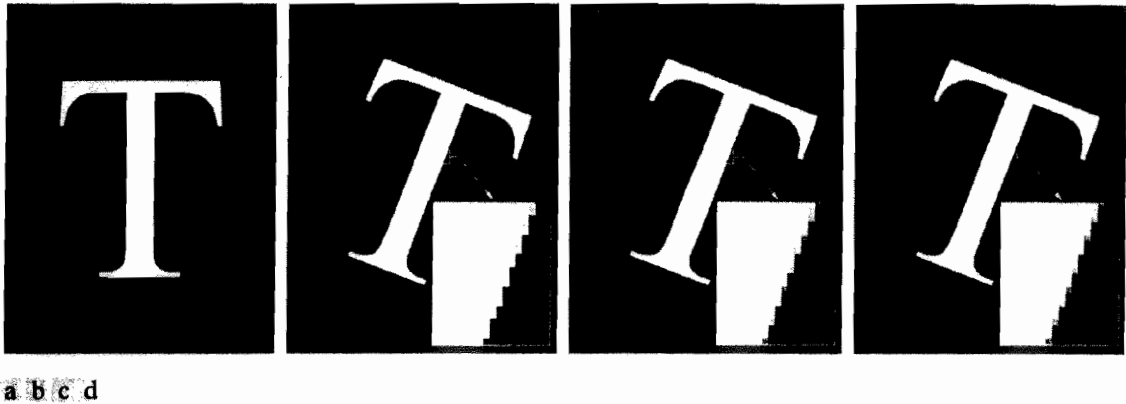
FIGURE 2.36 (a) A 300 dpi image of the letter T. (b) Image rotated 21^\circ using nearest neighbor interpolation to assign intensity values to the spatially transformed pixels. (c) Image rotated 21^\circ using bilinear interpolation. (d) Image rotated 21^\circ using bicubic interpolation. The enlarged sections show edge detail for the three interpolation approaches.
